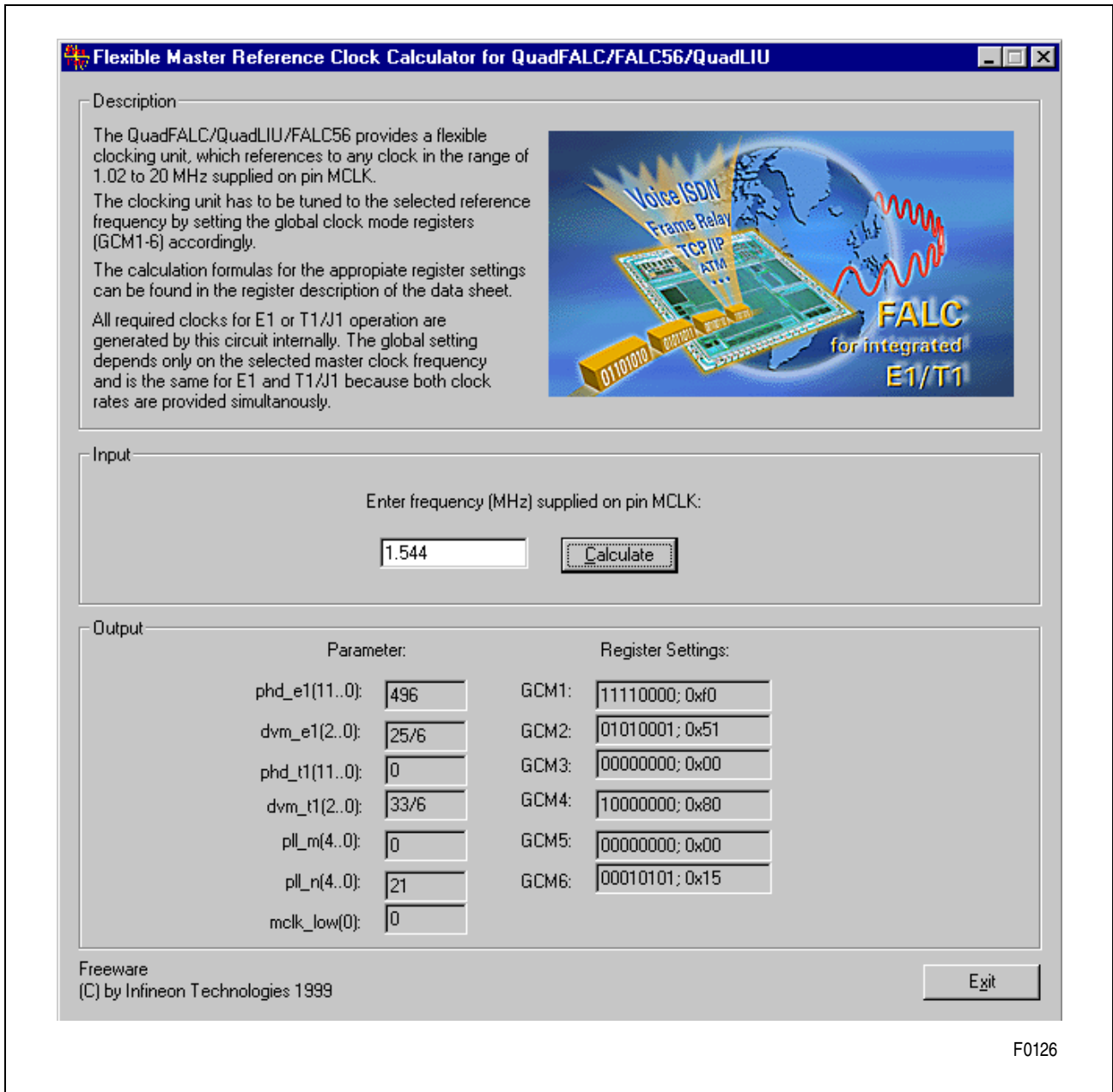
Figure 109 Master Clock Frequency Calculator
